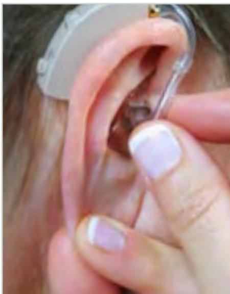
The volume control enables you to adjust the amount of amplification provided by the instrument. You may wish to change levels as you encounter different listening situations.
