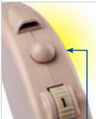
BTEs with a telecoil feature enable you to comfortably use the telephone without removing your instrument or earmold. The induction coil amplifies the signal emitted naturally from the telephone receiver.
