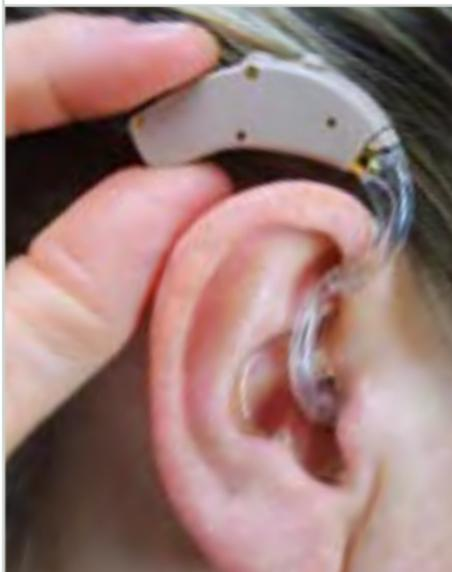
Carefully place the instrument behind your ear with the earhook and earmold tubing wrapped over the top.
