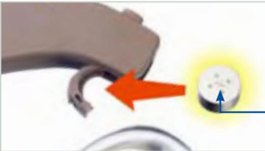
Place the new battery in the compartment with the plus (+) sign facing up.
