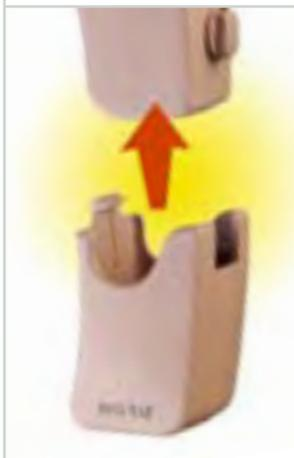
Your BTE is compatible with Direct Audio Input (DAI). This allows you to connect your instrument to another electronic sound source, such as a wireless FM system or audio and video equipment.
