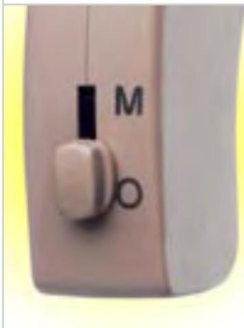
Your BTE has a two position switch to turn the instrument "on" and "off." To turn BTEs "on," move the switch to the "M" (microphone) position. To turn the instrument "off," move the switch to the "O" position.
