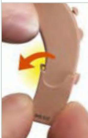
When the DAI module is attached, the instrument’s telephone coil is not active. Remove the module when using the telephone coil memory.
