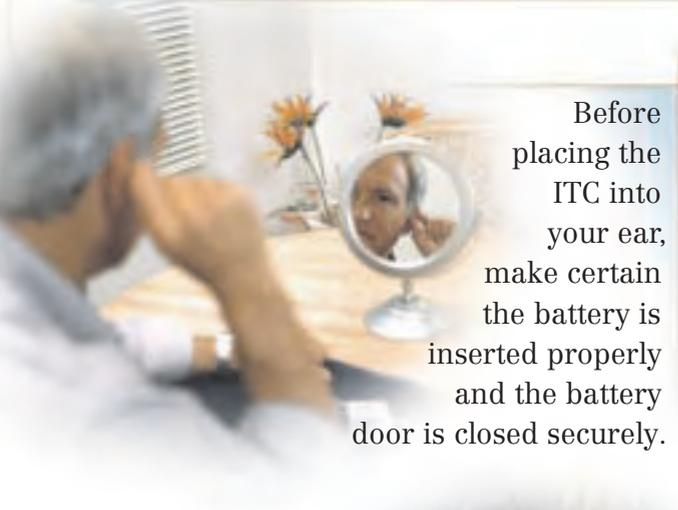
Before placing the ITC into your ear, make certain the battery is inserted properly and the battery door is closed securely.
