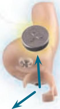
Remove the existing battery either by pushing it out the top of the door, or pulling it straight out.
